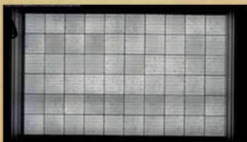
Before bending test, no micro cracks observed
